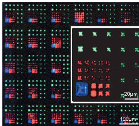
**Figure 2** PPL-generated multiplexed micropattern consisting of different types of fluorescently labelled phospholipids. With permission from [4]
