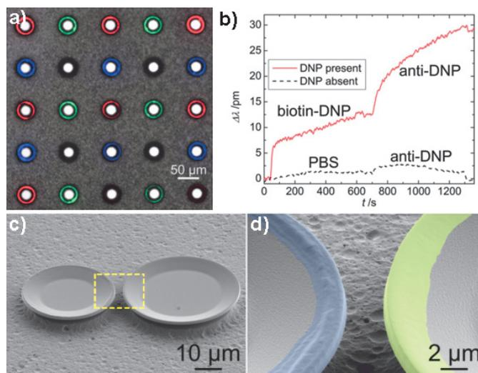
**Figure 6** a) Multiplex-functionalized goblet structures. b) Sensing of DNP antibodies. c) Electron microscopy image of two functionalized WGM structures and d) close-up with false colored lipid. Adapted with permission from [17, 18]
