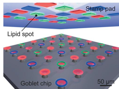
**Figure 5** Scheme of multiplexed WGM goblet functionalization by PPL generated stamp pad. With permission from [17]
