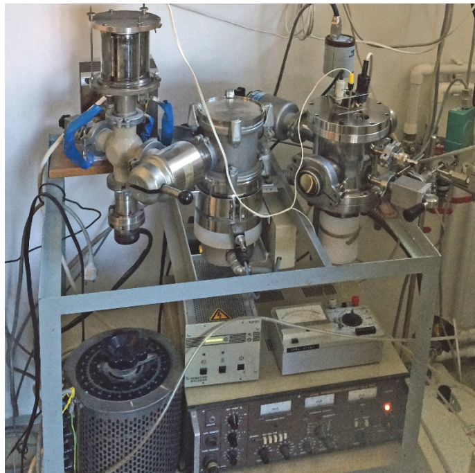
Figure 1 Reactive magnetron sputtering equipment
