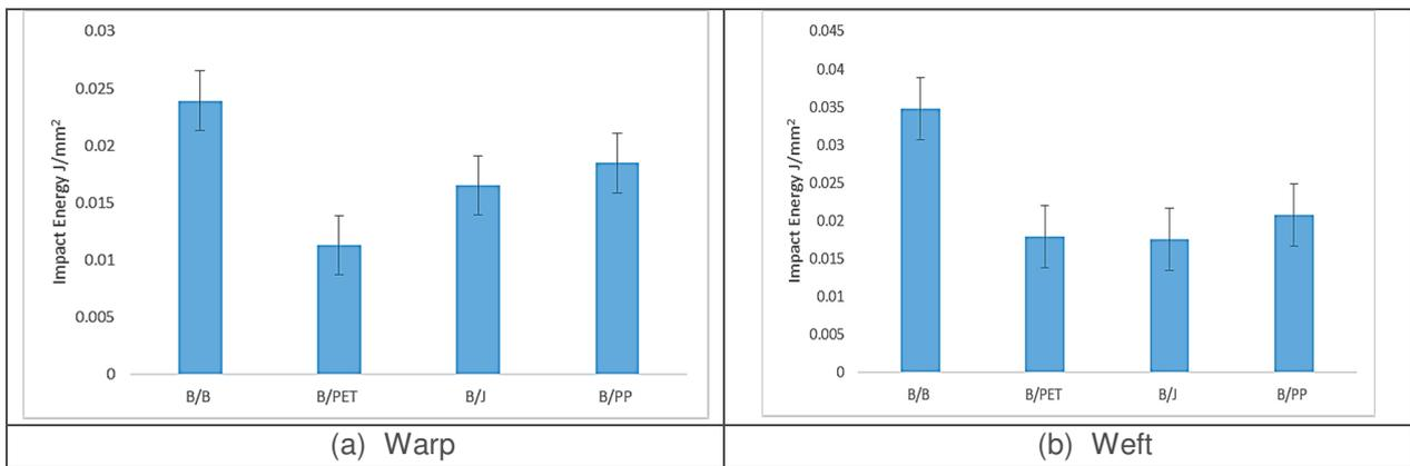
Figure 3 Impact strength of composites
