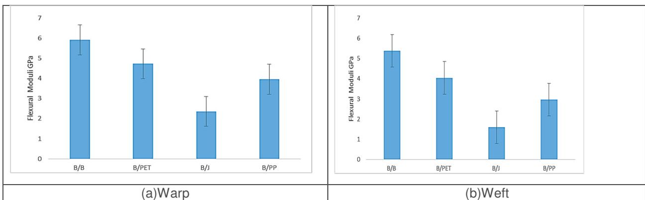
**Figure 2** Comparison of Flexural modulus of composites
