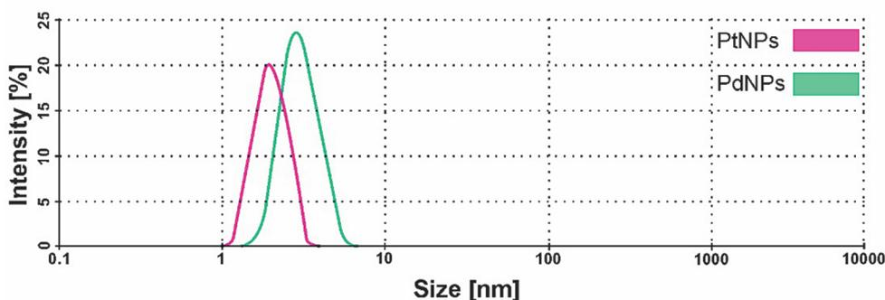
**Figure 2** Characterization of aqueous solutions with platinum and palladium nanoparticles by dynamic light scattering
