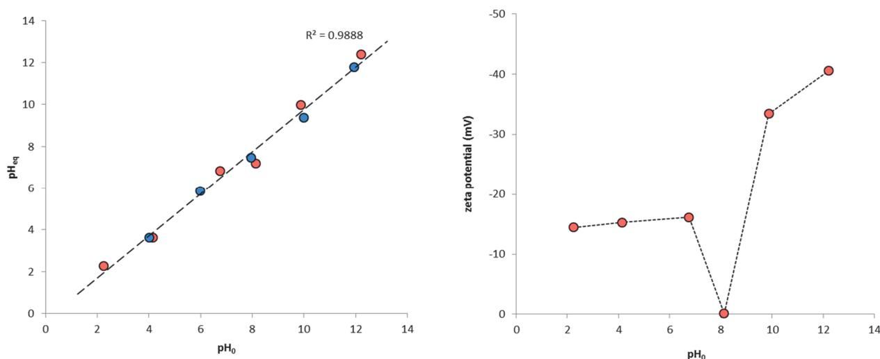
**Figure 1** Equilibrium pH values and zeta potential of humic fractions dissolved in buffer solutions (data obtained in ref. [16] are shown for comparison - blue circles)
