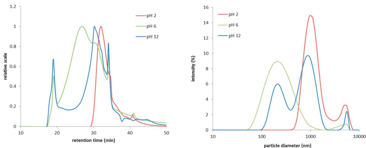
**Figure 3** Particle size distribution of humic fractions at pH 2, 6 and 12 determined by SEC (left) and DLS (right)
