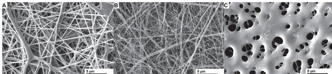
**Figure 2** SEM micrographs of electrospun substrates at the magnification of 10 000 (A) PCL, polymer concentration of 11 wt.%, applied voltage of 60 kV (B) PEG, polymer concentration of 9 wt.%, applied voltage of 40 kV, (C) PUR, polymer concentration of 18 wt.%, applied voltage of 60 kV
