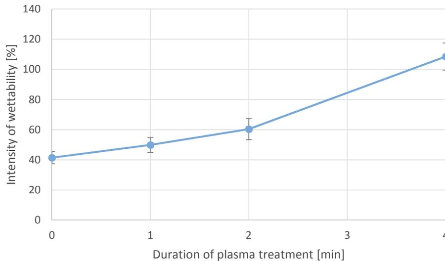
**Figure 2** Intensity of wettability of the modified carbon fibers
