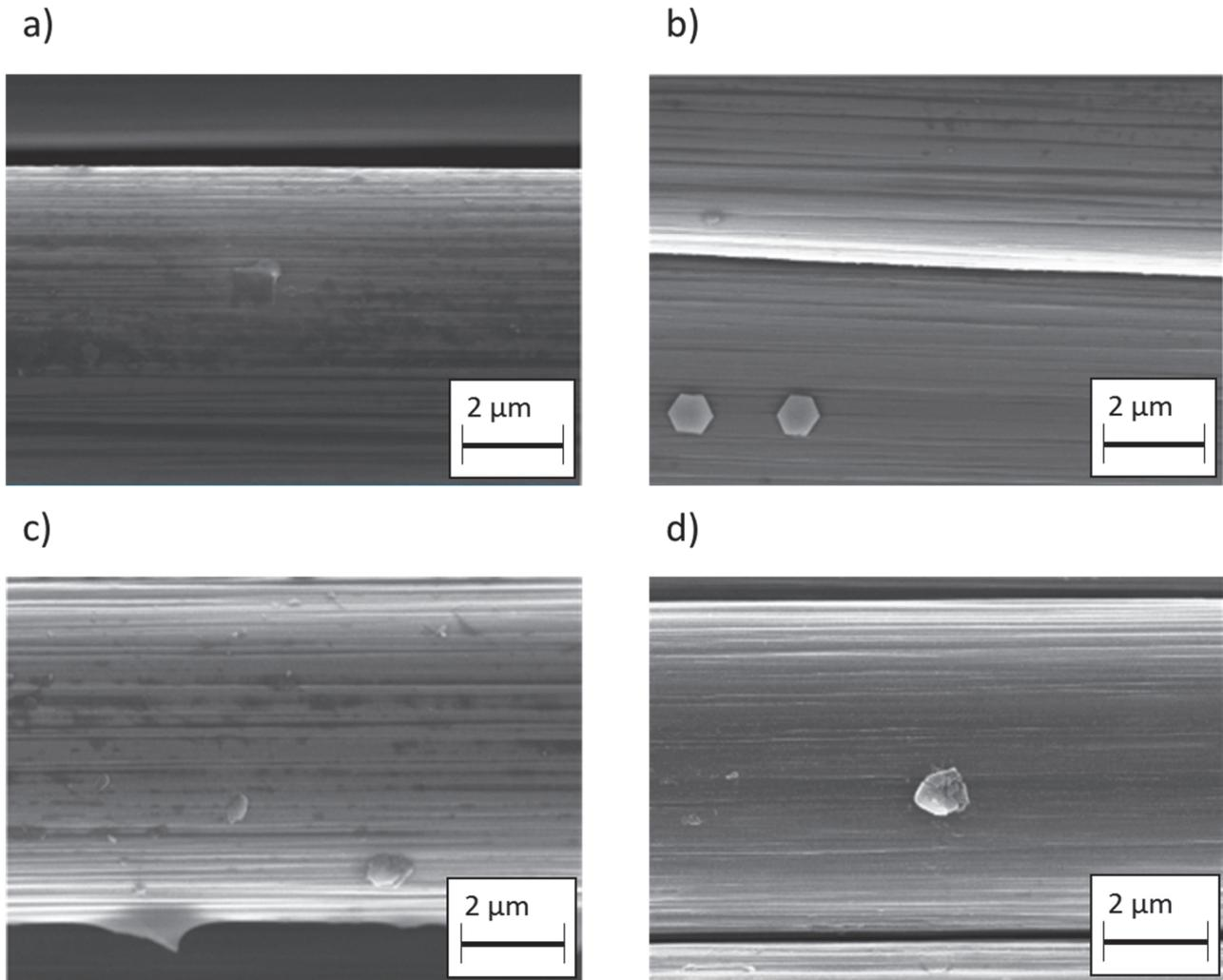
**Figure 1** SEM images of the modified carbon fibers as a function of treatment time: a - reference sample (CARBON 0'), b - 1 min. treatment (CARBON 1'), c - 2 min. treatment (CARBON 2'), d - 4 min. treatment (CARBON 4'), scale bar is 2 μm
