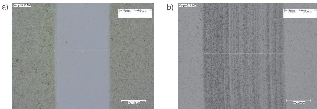
**Figure 8** Wear track of the (a) WC-CoCr and the (b) DLC coating respectively
