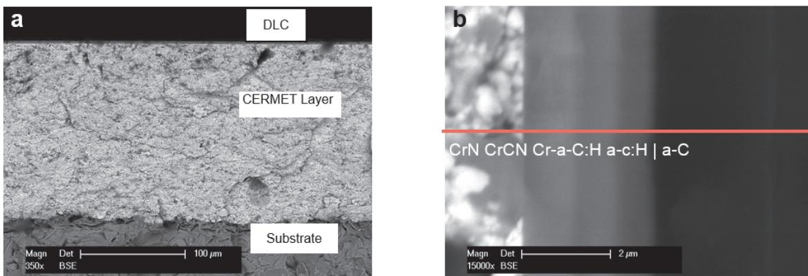
**Figure 4** SEM micrographs of the cross-sectioned DLC/WC-CoCr coatings systems as (a) overview and of the (b) EDX line scan
