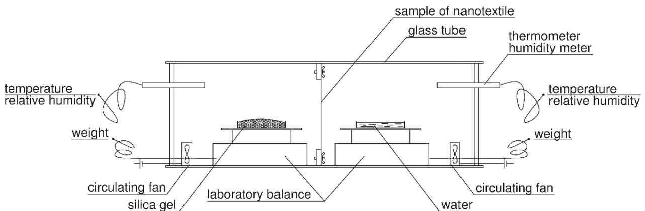
**Figure 4** Schematic representation of experimental device for measuring of diffusion properties of thin layers
