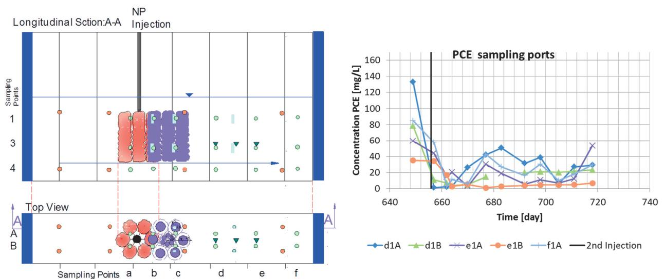
**Figure 5** Left - Position of PCE emplacement and NP injection for 1<sup>st</sup> and 2<sup>nd</sup> injection; right - Change of the PCE concentration in sampling ports at the downstream after 2<sup>nd</sup> injection
