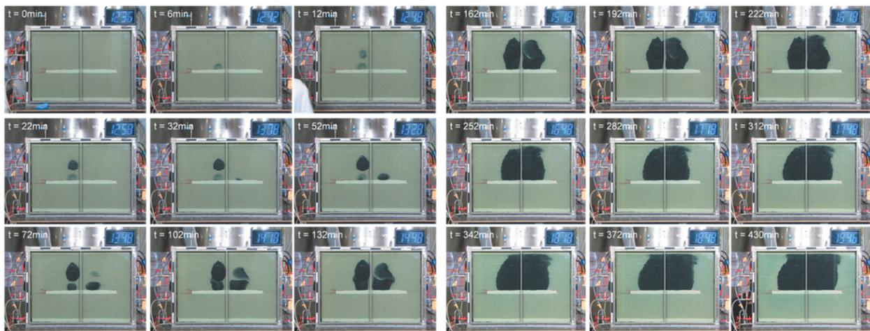
**Figure 3** Visualization of the 2D-migration experiment using NF 25S with the presence of a contaminant
