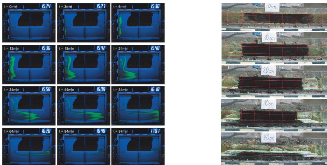
**Figure 4** left - Tracer test after nZVI injection; right - Disassembling of the experimental box layer by layer at the end of experiment
