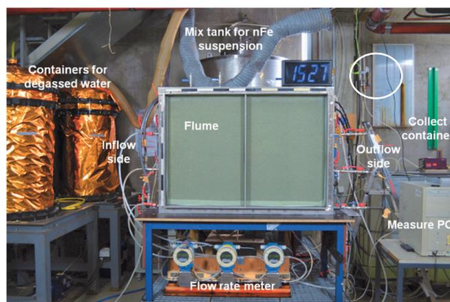
**Figure 1** 2-D experiment workstation at the VEGAS research centre
