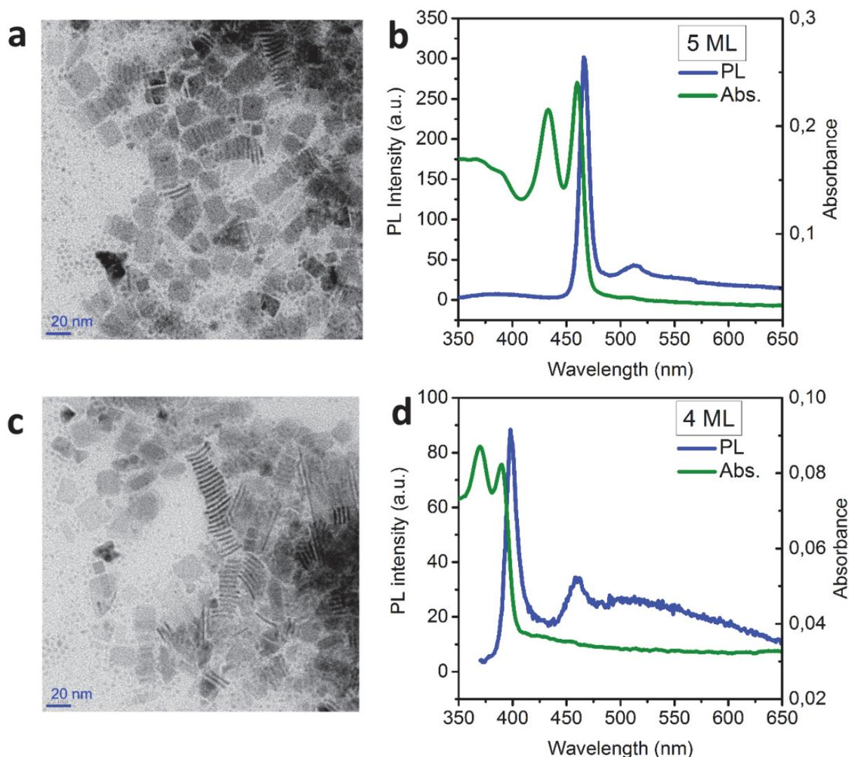
**Figure 1** TEM images, PL and Abs spectra of 5 ML (a, b) and 4 ML thick NPLs (c, d)
