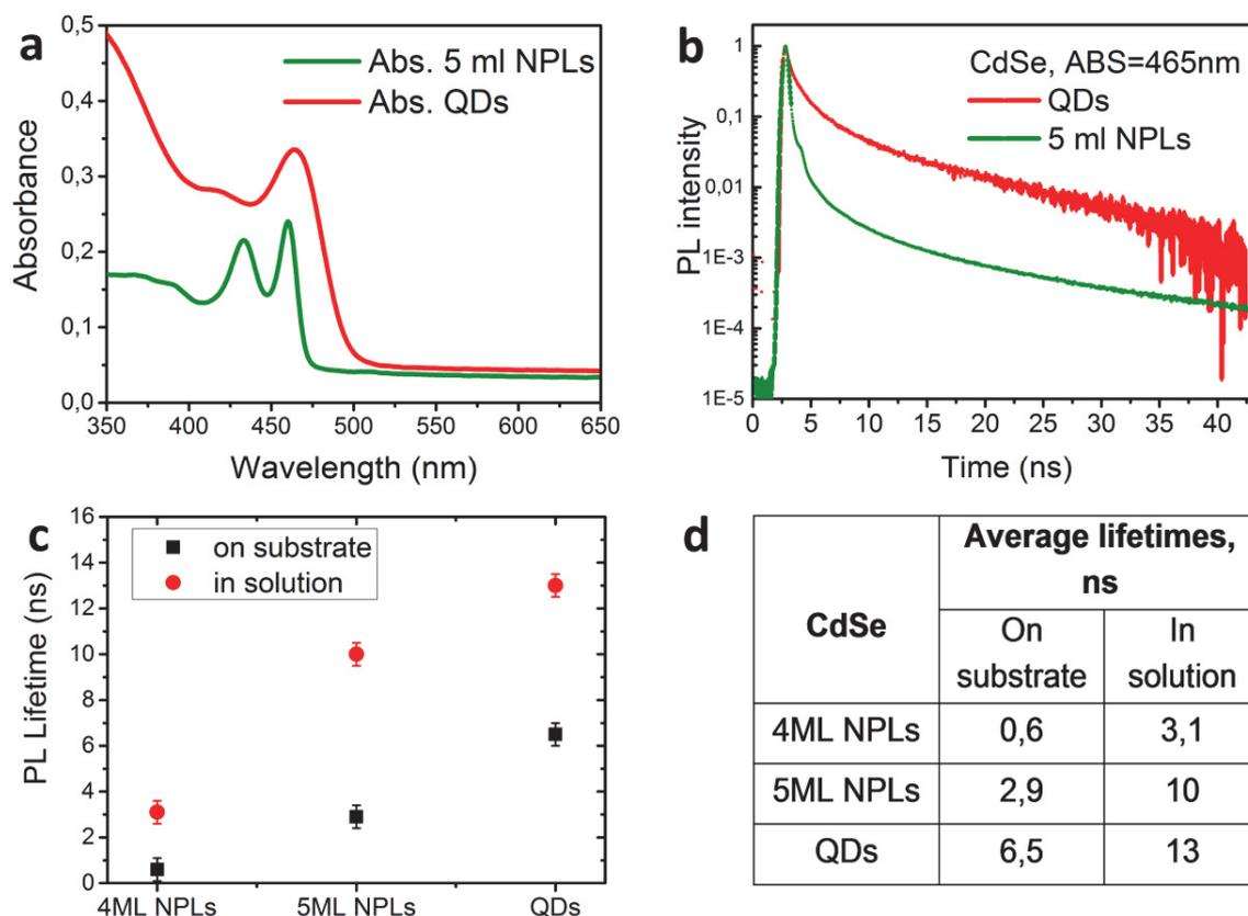
**Figure 3** Fluorescent lifetimes of NPLs and QDs: a) absorption spectra of 5 ML thick NPLs and QDs, b) PL decay curves of 5 ML thick NPLs and QDs: c) decay time dependence on the size and shape of NCs and d) table of measured numerical values for all NCs
