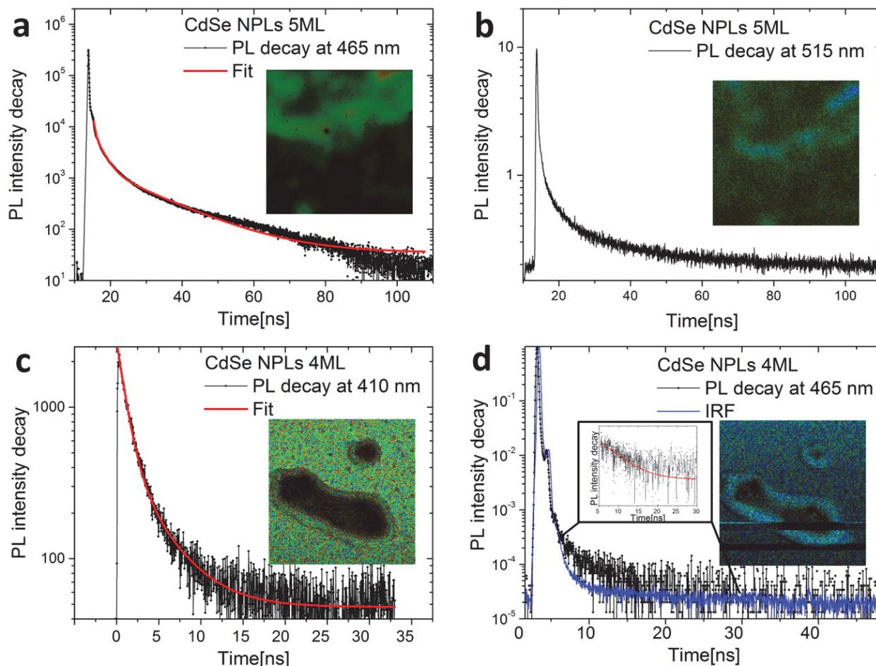
**Figure 2** PL decay curves at the main maximum and in the area of defect PL of 5 ML thick NPLs (a, b) and of 4 ML thick NPLs (c, d)
