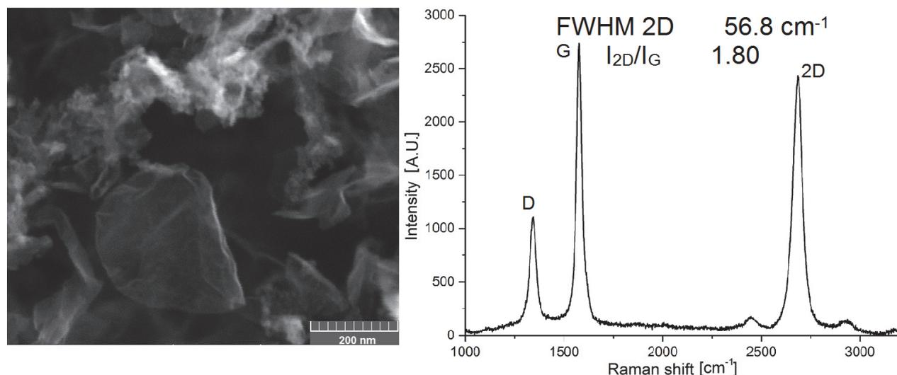
**Figure 2** (A) SEM image of prepared graphene flakes (GV2); (B) Raman spectroscopy of GV1
