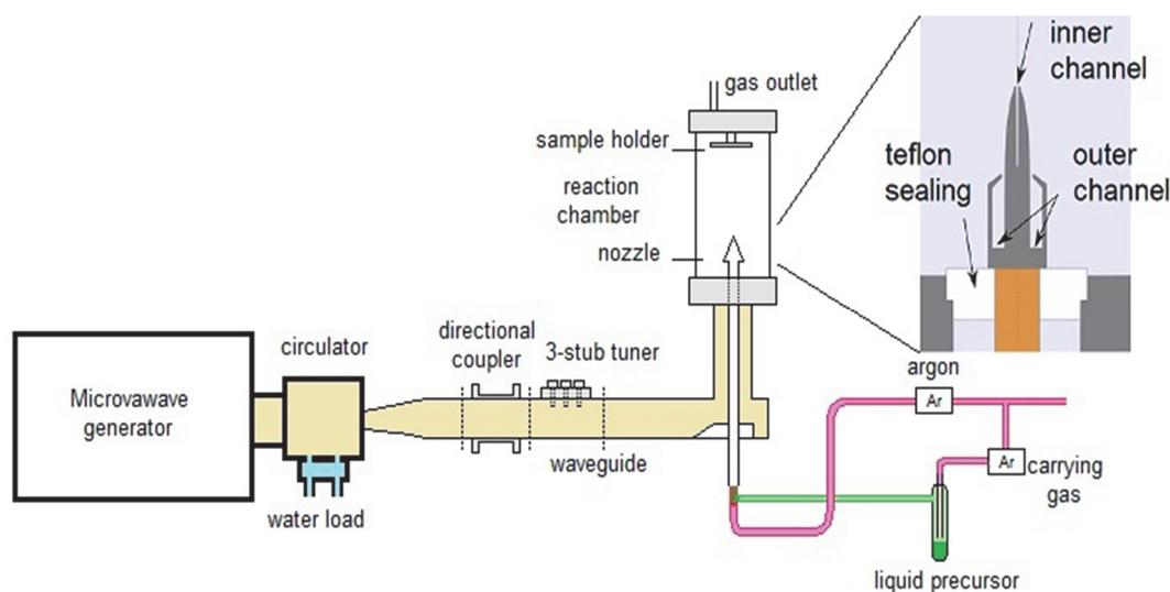
**Figure 1** Experimental setup for synthesis of graphene flakes by decomposition of ethanol precursor in microwave plasma torch discharge with a detailed view of the nozzle [12]
