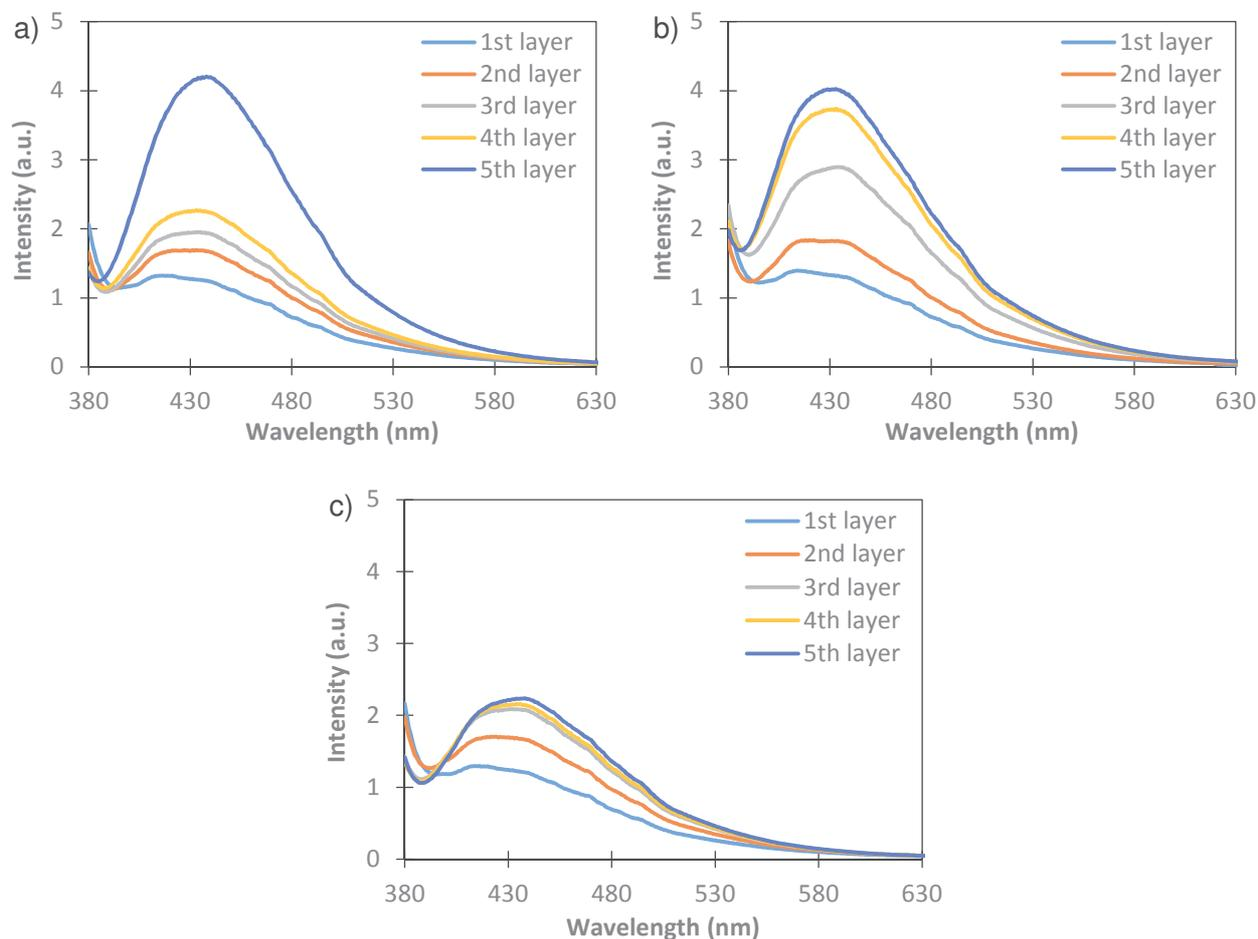
**Figure 4** Fluorescence spectra of ZnO:Cu in a) CMC, b) PVP, and c) 2HEC polymeric binders after deposition on Standard IGT paper
