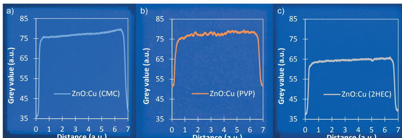
**Figure 3** Printed samples of ZnO:Cu in a) CMC, b) PVP, and c) 2HEC binder with averaged profile plots of the samples as representation of the homogeneity of deposited films
