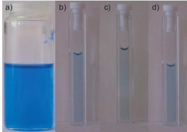
**Figure 1** Photographs of a) ZnO:Cu colloid and its ink compositions with binders b) CMC, c) PVP, and d) 2HEC
