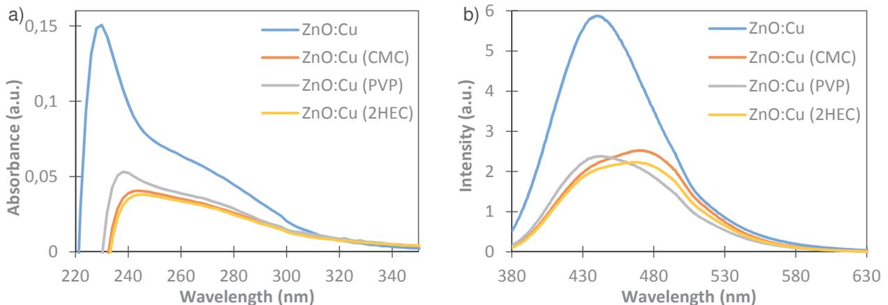
**Figure 2** a) UV-Vis spectra and b) fluorescence spectra of starting colloid ZnO:Cu and its ink compositions with polymeric binders
