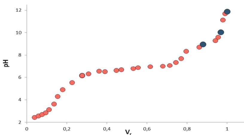
**Figure 1** Measurement of pH during precipitation synthesis, emphasized are samples 1, 2 and 3 [7]
