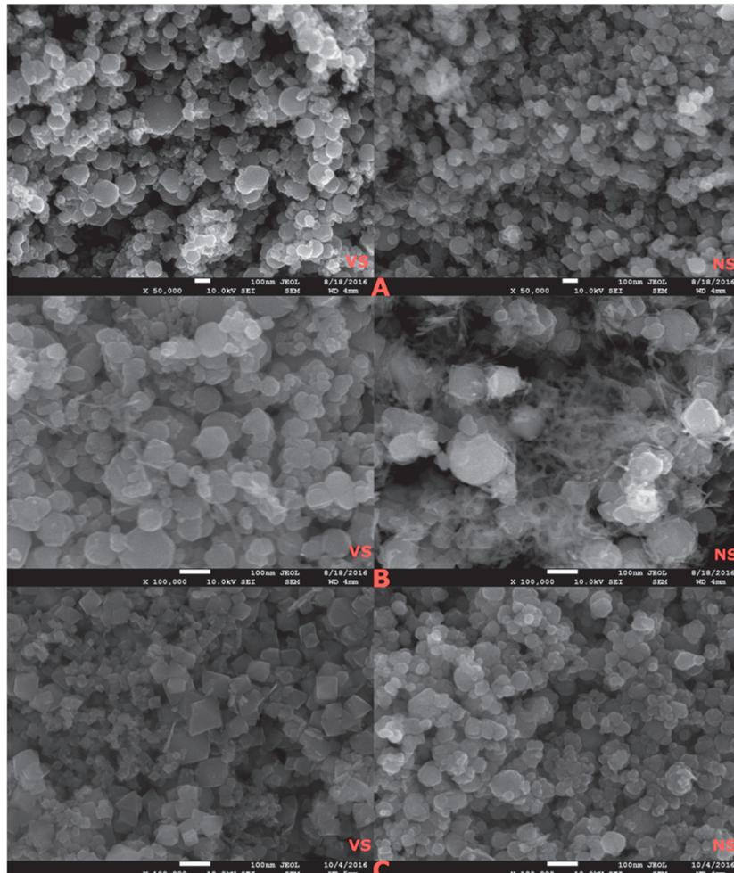
**Figure 5** Analysis of vigorously stirred and non-stirred samples with various pH during precipitation
