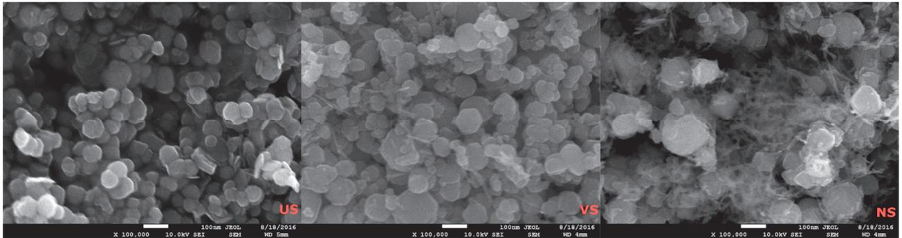
**Figure 4** Different stirring conditions applied during precipitation at 60°C (US - ultrasonified, VS - vigorous stirring, NS - non-stirred)
