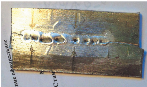
Figure 2 Welded specimen top view (arrows pointing on CNTs placement)
