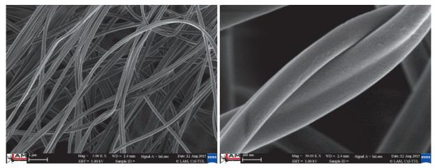
Fig. 2 SEM images of the smooth fibres after the electrospinning process
