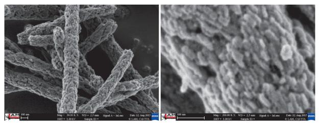
**Fig. 3** TiO<sub>2</sub> fibres after the calcination at 600 °C. The porous surface and nanocrystal structure are clearly visible in the detailed image. The size of anatase crystals is in a range of tens of nm
