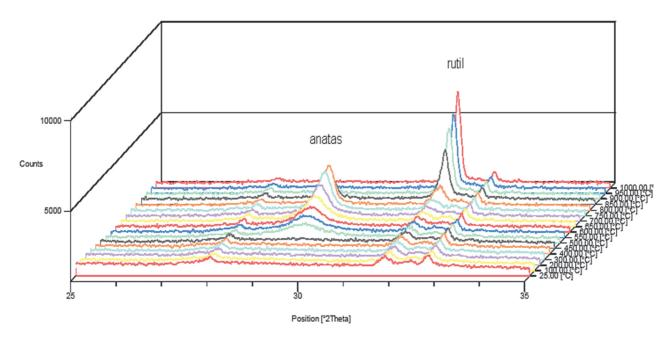
**Fig. 1** XRD curves shoving the effect of temperature on the crystal structure of TiO<sub>2</sub> nanofibers. At low temperatures the spinned fibres are almost amorphous. Anatase appears in the structure at 500 °C and its amount increases up to 700 °C. Above 700 °C the anatase transforms to rutile phase
