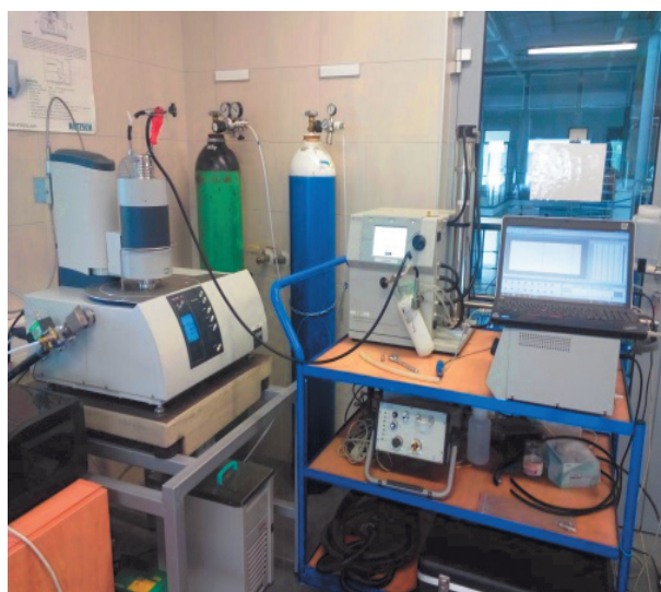
Fig. 1 Experimental setup. TGA + SMPS
