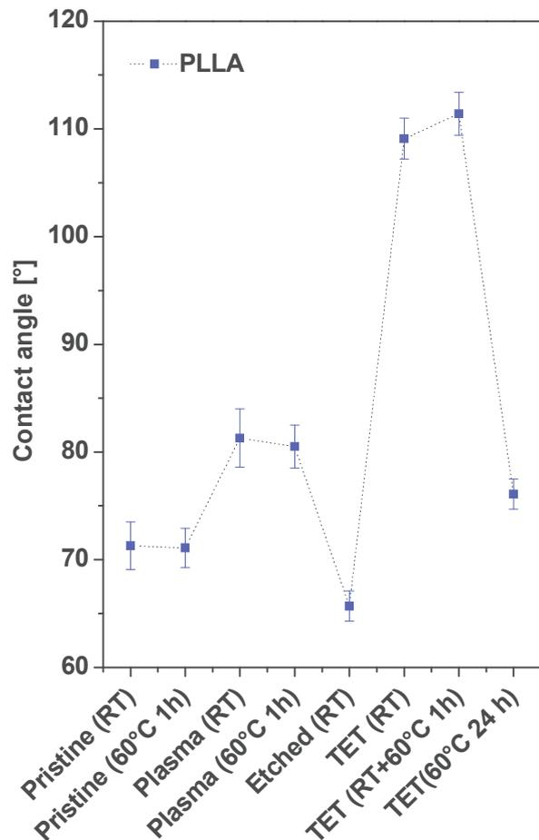
**Fig. 3** Water contact angle measured on various PLLA samples (with and without thermal stress): pristine (pristine), plasma treated (plasma), etched in water solution of hydrochloric acid (etched) and CNPs grafted (TET)
