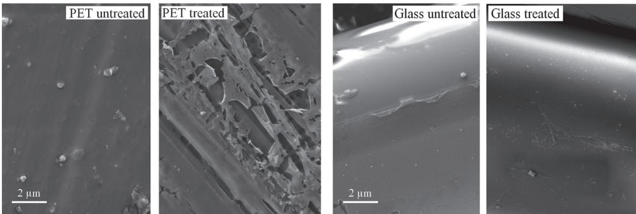
Fig. 3 SEM images of PET and glass fibers before and after the oxygen plasma treatment
