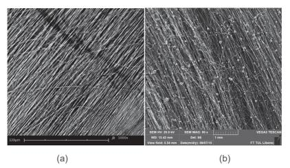
Fig. 3 Image analysis: (a) PVA layer, (b) PVDF layer
