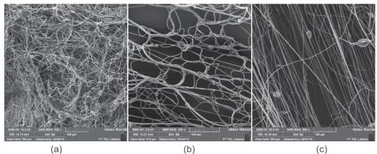
Fig. 4 Image analysis: (a) PVDF/PEO Nanospider layer, (b) PVDF/PEO layer from original device (c) PVDF/PEO from the novel device
