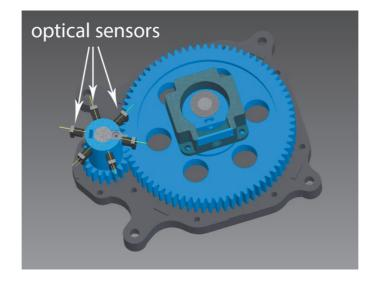
Fig. 2 Position of optical sensors
