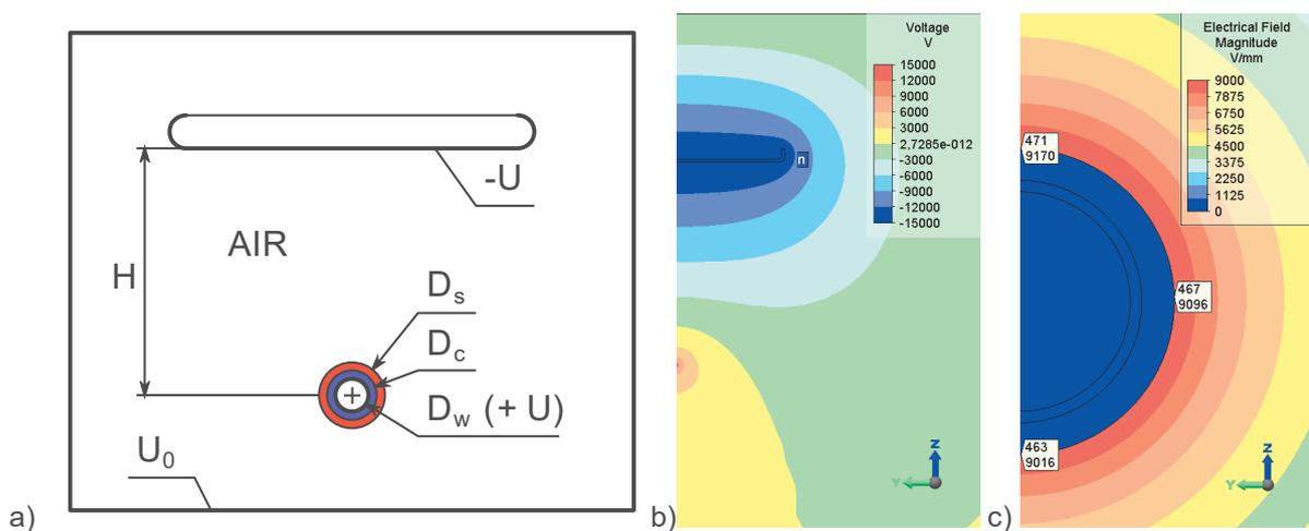
**Fig. 2 a)** The 2-D wire spinner model layout in the software environment Autodesk Simulation Mechanical. **b)** Results: Voltage distribution (half-model) **c)** Results: Electric field strength (detail of the wire electrode)
