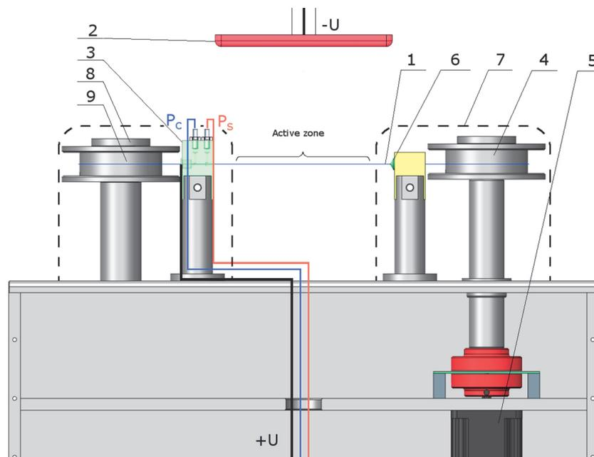
**Fig. 1** The scheme of the wire spinner, 1: Wire electrode (+U), 2: collector (-U), 3: Polymer solution (s) dosing cartridge, 4: Driven pulley, 5: Step motor, 6: Wire guide, 7: Covers, 8: Friction brake, 9: Free pulley
