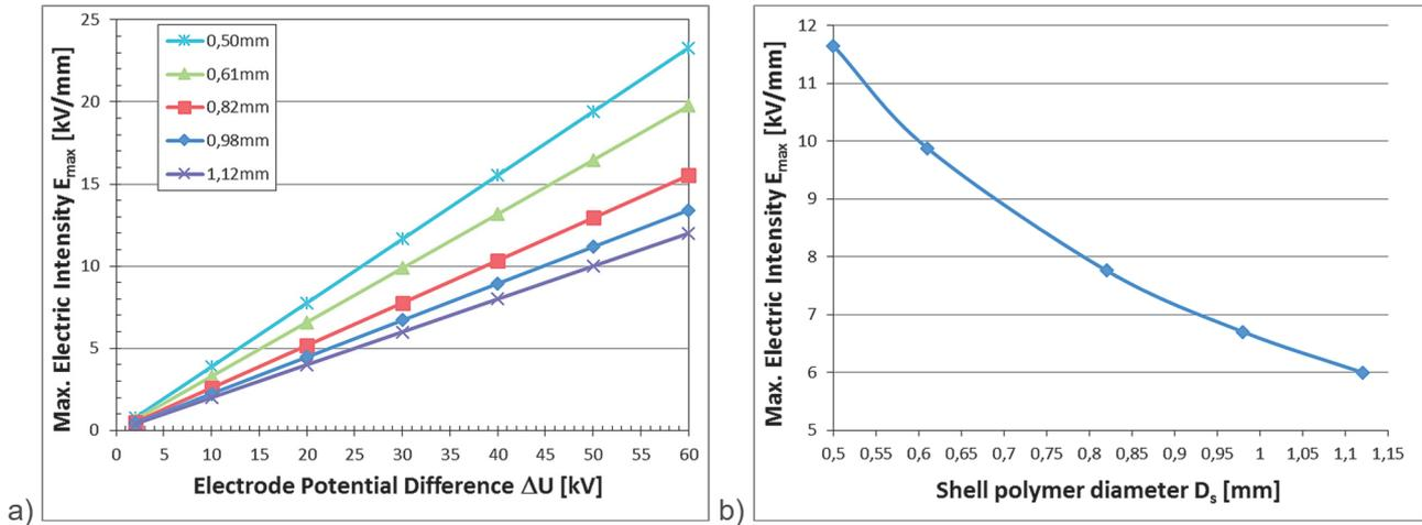
**Fig. 3** Results of the electrostatic analysis **a)** Dependency of Max. Electric Intensity  $E_{max}$  on the electrode potential difference  $\Delta U$  (under constant electrode distance  $H=150$  mm) **b)** Dependency of Max. Electric Intensity  $E_{max}$  on the shell polymer diameter  $D_s$  ( $H=150$  mm,  $\Delta U=30$  kV)
