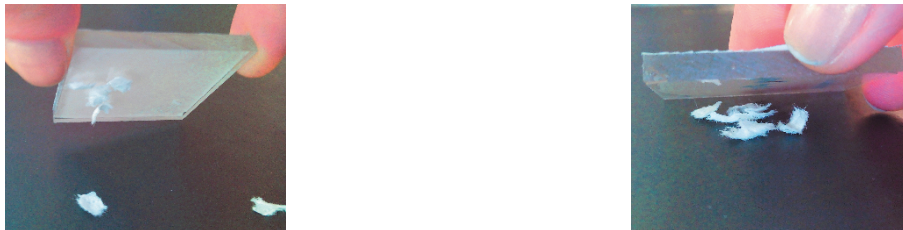
Fig. 1 The antistatic effect of the impregnating emulsion (left) untreated sample, (right) treated sample
