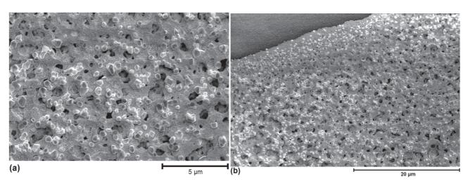
Fig. 1 SEM microscopy of the silver ink structure on the PET substrate. (a) detail (scale of 5  $\mu$ m) (b) overview (scale of 20  $\mu$ m)
