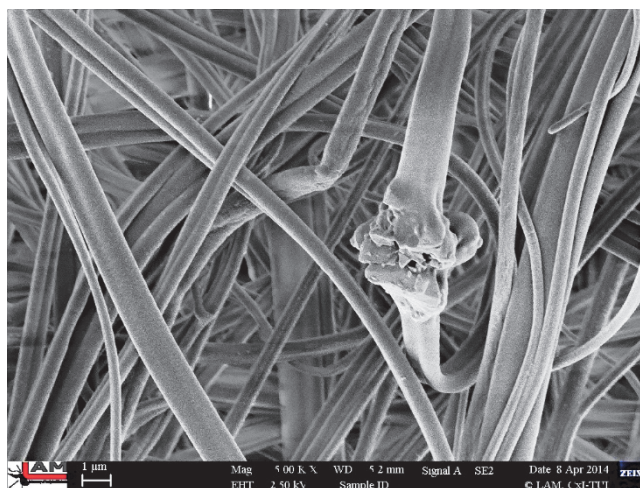
Figs. 7, 8 SEM image of PVB nanofibers with Bi 3+ tungstates
