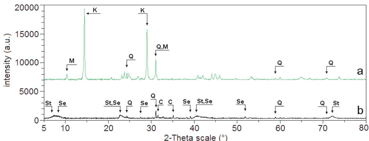
**Fig. 1** XRPD patterns of pure kaolin KKAF (a) and ghassoul (b) used for the preparation of nanocomposites. C - clinoenstatite, K - kaolinite, M - muscovite, Q - quartz, Se - sepiolite, St - stevensite
