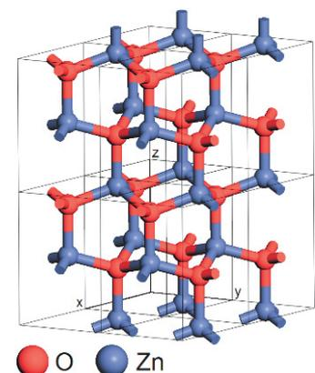
**Fig. 3** Hexagonal (wurtzite) structure of ZnO having lattice parameters:  $a = 3.24927$  Å,  $b = 3.24927$  Å,  $c = 5.20544$  Å,  $\alpha = 90$  °,  $\beta = 90$  °,  $\gamma = 120$  °
