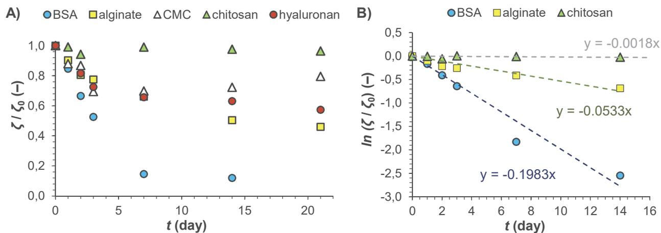
**Fig. 3** Results zeta potential measurements after the application of first order kinetic A) the time development of zeta potential values, B) linearization of selected time developments of zeta potential values
