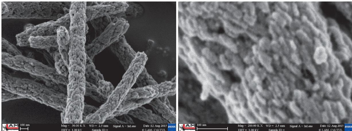
**Fig. 3** TiO<sub>2</sub> fibres after the calcination at 600 °C. The porous surface and nanocrystal structure are clearly visible in the detailed image. The size of anatase crystals is in a range of tens of nm
