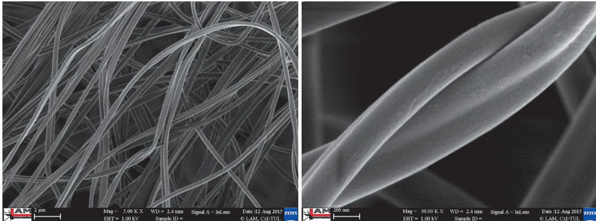
**Fig. 2** SEM images of the smooth fibres after the electrospinning process
