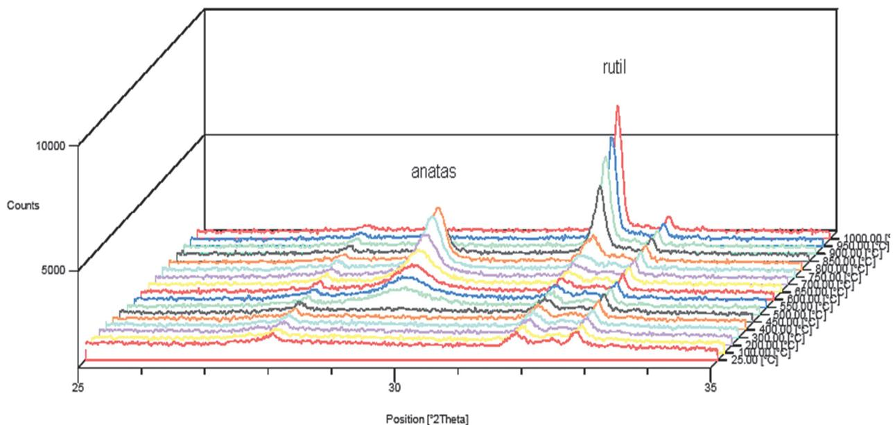
**Fig. 1** XRD curves showing the effect of temperature on the crystal structure of TiO<sub>2</sub> nanofibers. At low temperatures the spinned fibres are almost amorphous. Anatase appears in the structure at 500 °C and its amount increases up to 700 °C. Above 700 °C the anatase transforms to rutile phase
