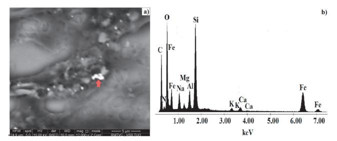
**Fig. 4** SEM image of a cluster of particles containing iron detected in the lung tumor tissue sample (a) with the corresponding EDX spectrum (b)
