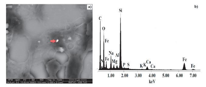
Fig. 3 SEM image of particle containing iron detected in the lung tumor tissue sample (a) with the corresponding EDX spectrum (b)
