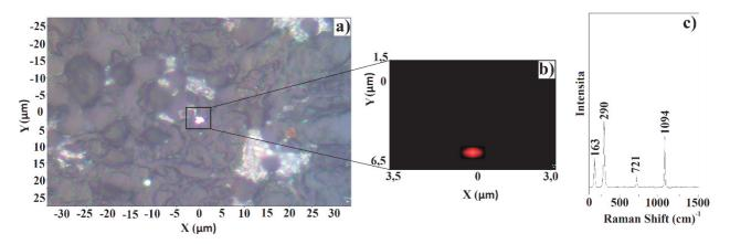
**Fig. 1** Raman spectral map of the selected area of the lung cancer tissue, where a) light microscopy image of the tissue with the selected area, b) the spectral map of the selected area (red - siderite, black - surrounding tissue) and c) the measured Raman spectrum of siderite
