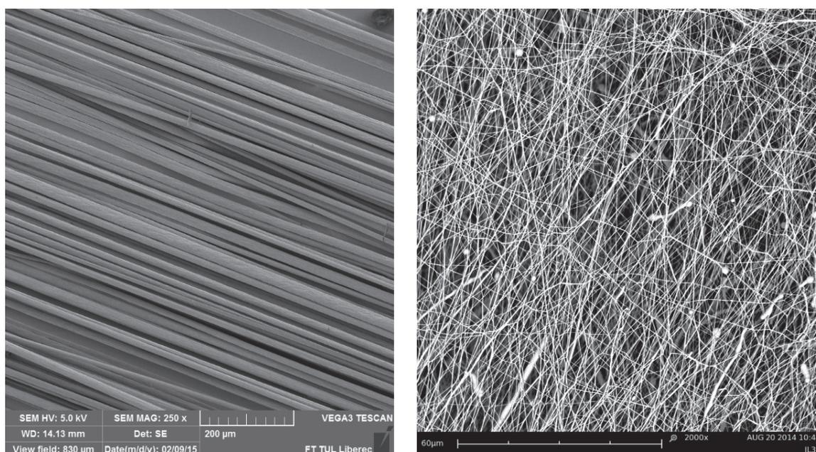
**Fig. 1** SEM images of polycaprolactone fibers made by drawing (*left*) and electrospinning technique (*right*)
