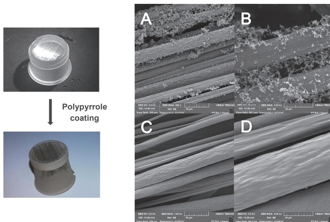
**Fig. 2.** (left) PCL fibers made by drawing technique tailored on the PMMA circllet, (right) SEM images of PCL fibers coated by PPy layer (a, b) clusters formation (c, d) optimized reaction conditions
