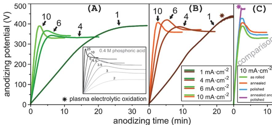
**Fig. 1** Potential-time responses of (A) as rolled, (B) vacuum annealed aluminium foils during galvanostatic anodizing in 0.05 M citric acid. (C) shows the comparison of galvanostatic anodization at 10 mA·cm<sup>-2</sup> for various foils. The inset shows a classical galvanostatic anodizing behaviour of aluminium foil in 0.4 M phosphoric acid acid
