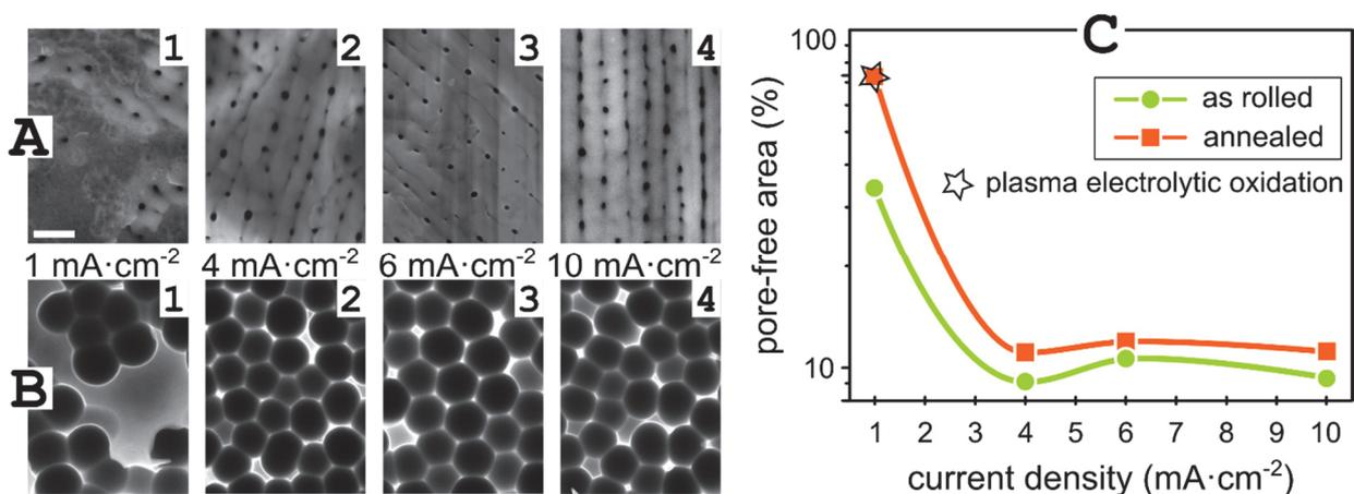
**Fig. 2** SEM images of the as-rolled foils anodized as in **Fig. 1A** before (row A) and after (row B) selective alumina dissolution. The graph (C) shows the pore-free area vs. anodized current density curves (as measured) for the as-rolled and annealed foils anodized as in **Fig. 1A-B**. The scale bar is  $1 \mu\text{m}$
