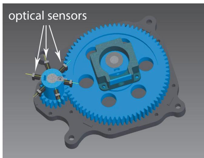
**Fig. 2** Position of optical sensors
