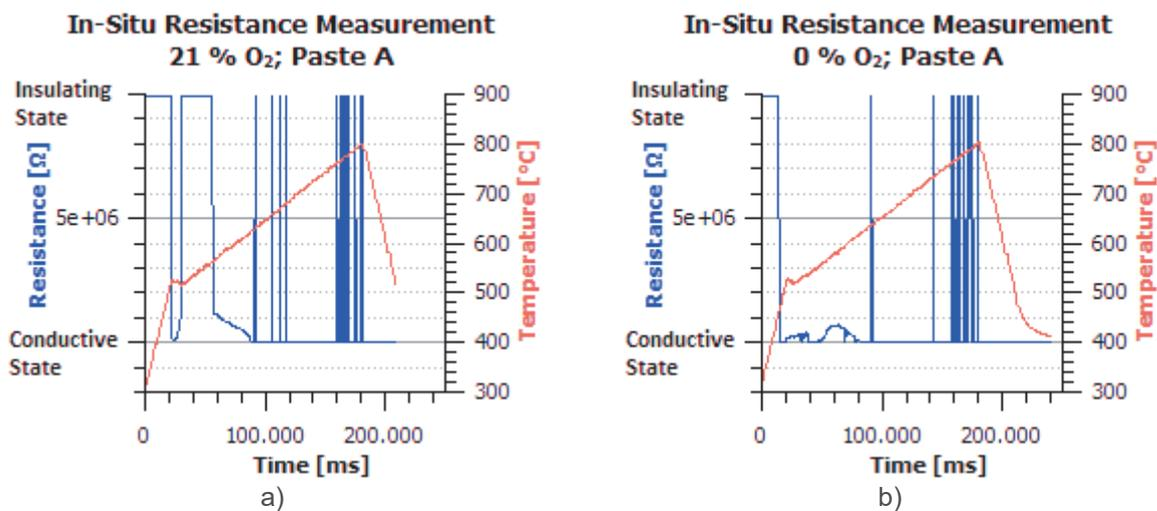
**Fig. 3** The dependence of resistance on the temperature and the content of O<sub>2</sub> for the paste A
