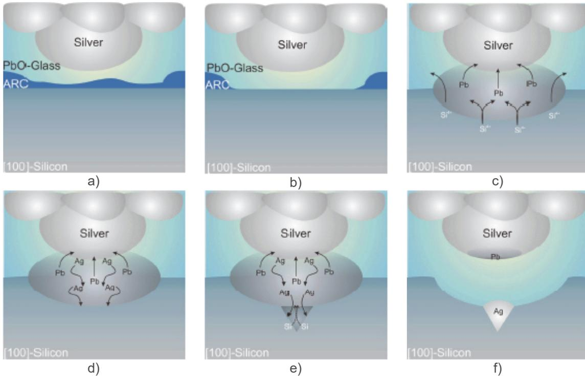
**Fig. 1** Simplified model of contact formation: a) schematic cross section of Ag thick film paste on [100] Si after combustion of organics; b) glass etches through SiN<sub>x</sub> layer; c) redox reaction between Si and glass, lead (Pb) is formed; d) liquid Pb starts to melt Ag; e) Ag - Pb melt reacts with Si, inverted pyramids are formed; f) on cooling down Ag recrystallises on (111)-Si planes [5]
