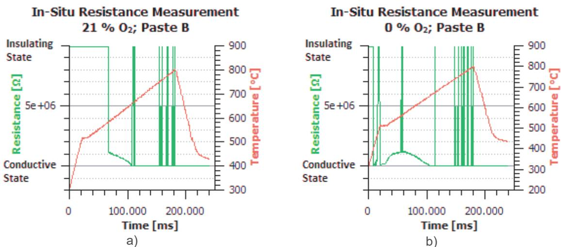
**Fig. 4** The dependence of resistance on the temperature and the content of O<sub>2</sub> for the paste B
