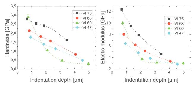
Fig. 7 (on the left) The dependence of the hardness on the indentation depth for coatings on polycarbonate substrates. (on the right) The dependence of elastic modulus on the indentation depth for coatings on polycarbonate samples. The deposition conditions of the selected coating are given in Table 1.
