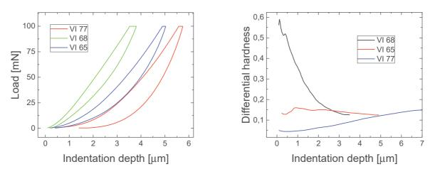
Fig. 6 (on the left) Examples of loading/unloading curves for coatings deposited on polycarbonate samples. (on the right) Examples of differential hardness (in GPa) dependence for coatings on polycarbonate samples. The differential hardness was calculated as the derivative of the load function with respect to the increasing contact area. The deposition conditions of the selected coating are given in Table 1.
