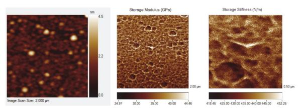
Fig. 4 Example of 2x2 μm<sup>2</sup> topography image (on the left) of nanocomposite film [RMS (root mean square roughness) = 0.9 nm, Ra (average roughness) = 0.6 nm], storage modulus map on the same area (in the middle) and detail of storage stiffness map (on the right) on area of 500x500 nm<sup>2</sup>
