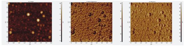
**Fig. 3** Example of topography image (on the left) obtained using AFM imaging of nanocomposite film, map of the work of adhesion in mJ/m<sup>2</sup> (in the middle) and the stiffness map in N/m (on the right)
