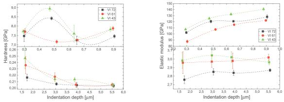
Fig. 5 (on the left) Examples of the hardness dependences on the maximum indentation depth for films deposited on silicon substrates (top) and on polycarbonate substrates (bottom). (on the right) The dependence of elastic modulus on the maximal indentation depth for coatings on substrates (top) and on polycarbonate substrates (bottom). The dashed lines are only guides for eyes. The coatings deposition conditions are given in the Table 1.
