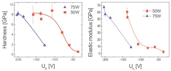
Fig. 2 The dependence of the hardness (on the left) and the elastic modulus on the bias voltage (on the right) for to applied powers 50 and 75 W
