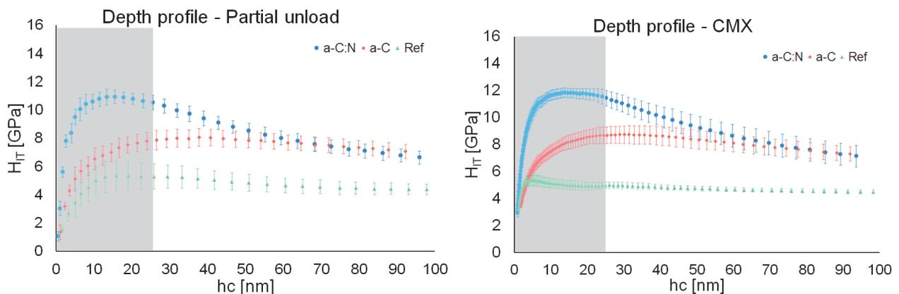
**Fig. 6** Indentation hardness, the values of  $H_{IT}$  are calibrated from depths of  $h_c = 25\text{ nm}$ . The grey rectangle demarcates uncalibrated data
