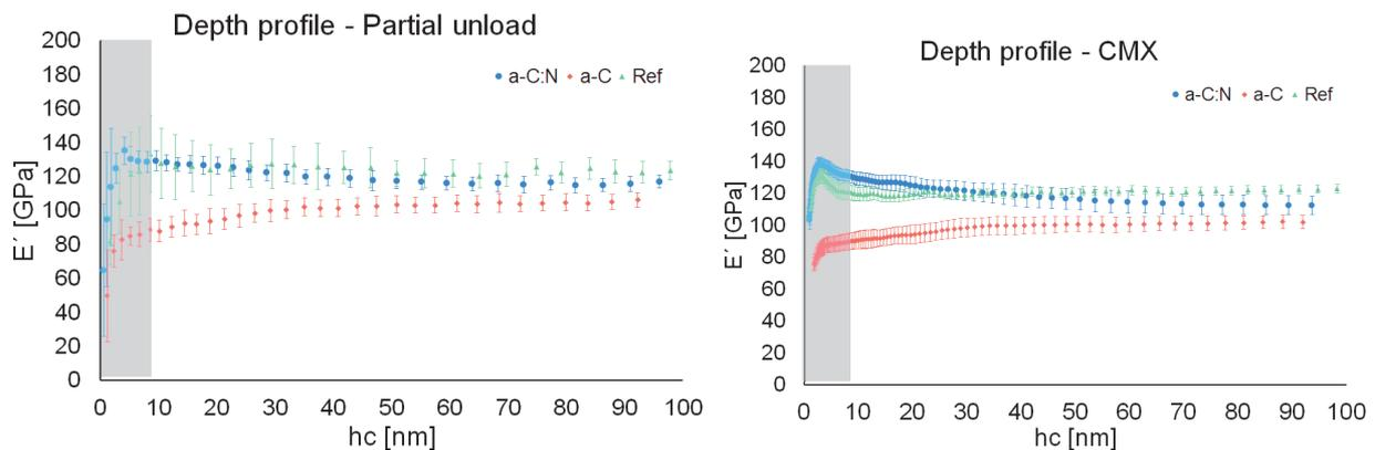
**Fig. 5** Depth profiles of the storage modulus. Left - Partial unload results. Right - Continuous Measurement of X. Values of  $E'$  are calibrated from depths of  $h_c = 8\text{ nm}$ . The grey rectangle demarcates uncalibrated data
