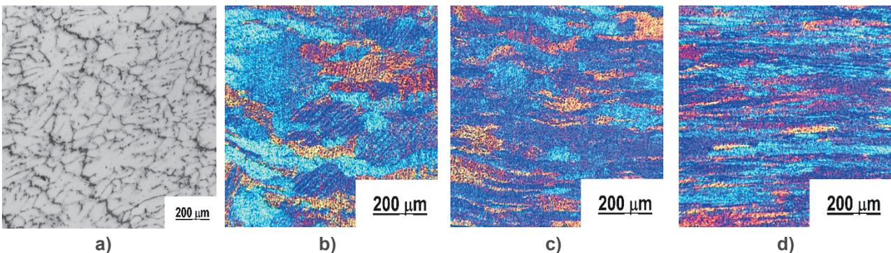
**Fig. 3** Structure of the EN AW 3003 alloy, a) initial state, b) after 2<sup>nd</sup> pass, c) after 4<sup>th</sup> pass, d) after 6<sup>th</sup> pass
