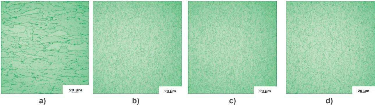
**Fig. 2** Structure of the steel DC 01, a) initial state, b) after 2<sup>nd</sup> pass, c) after 4<sup>th</sup> pass, d) after 6<sup>th</sup> pass
