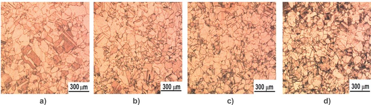
**Fig. 4** Structure of the brass EN CW 508L, a) initial state, b) after 2<sup>nd</sup> pass, c) after 4<sup>th</sup> pass, d) after 6<sup>th</sup> pass
