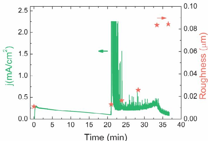
**Fig. 4** The current density - time response during potentiodynamic anodizing (green curve, left axis) with notes for the surface roughness values measured for samples anodized to corresponding potentials (red stars, right axis)
