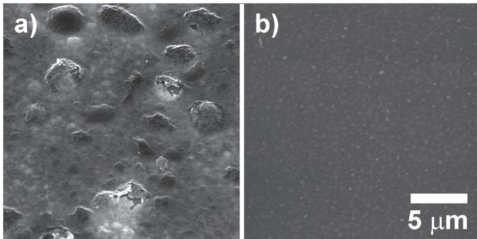
**Fig. 3** (a) sample MS 1 after anodizing - a serious surface damage of the anodic film is clearly visible, (b) sample IBD 2 after anodizing - the surface of the anodic film remains relatively flat without visible damages. Both images were recorded at a 40° tilt to the substrate. The scale bar is for both images.
