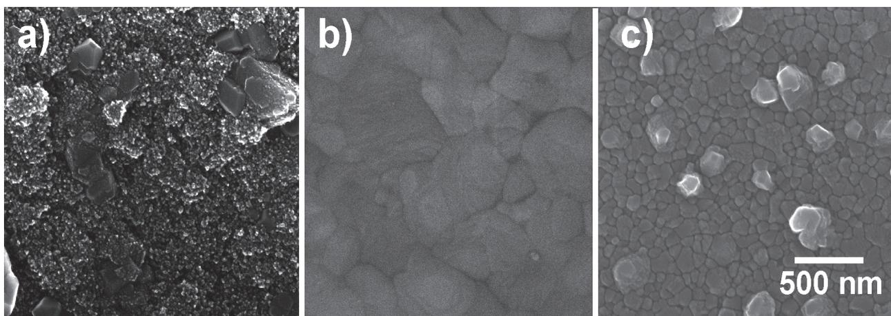
**Fig. 1** SEM images of aluminium thin film deposited by (a) an ion beam assisted deposition (sample IBD 3), (b) a magnetron sputtering (sample MS 1) and (c) a thermal evaporation (sample TE 2). The variety of surface structure and morphology of the Al films deposited by various techniques is clearly visible. The scale bar is valid for all 3 images
