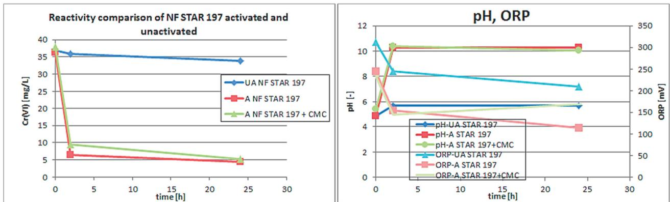
**Fig. 3** Results of the batch test of STAR 197 with and without CMC treatment
