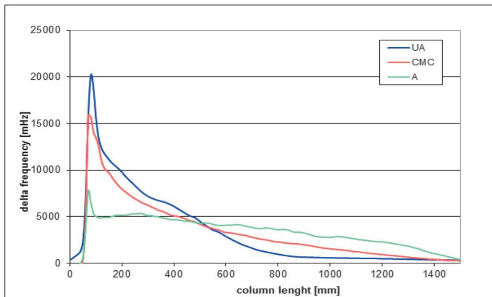
**Fig. 4** Longitudinal profile of Fe<sup>0</sup> in columns after 2 hours of injection for STAR 197 in different states of preparation, unactivated (UA), activated (A) and modified by CMC (CMC)
