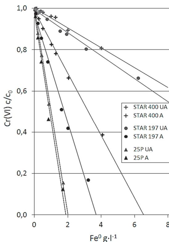
**Fig. 2** Concentration tests of activated and unactivated NF 25P, STAR 400 and 197
