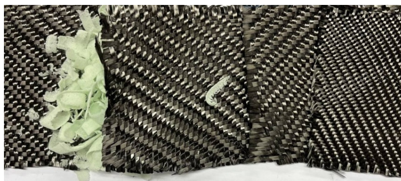
Figure 3 Schematic of the sandwich structure with a recycled PU chip core between carbon/epoxy face sheets
