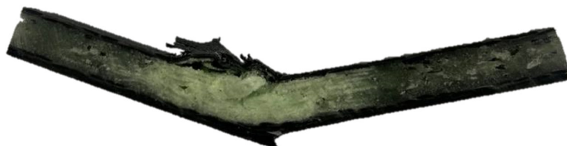
Figure 5 Typical post-test condition of the specimen indicating core damage and face-sheet cracking
