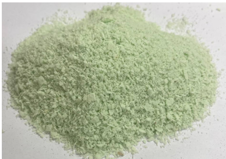
Figure 2 Chips generated during machining of the PU modelling board
