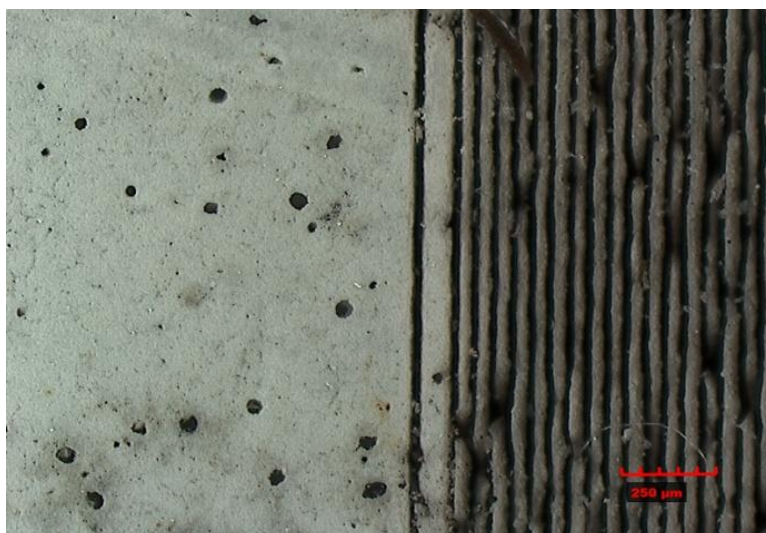
Figure 3 Topcoat of the masking coating system before and after laser cleaning (variant A)
