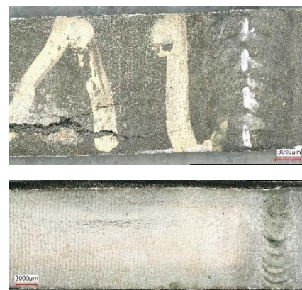
Figure 5 Creep damage on the outer (above) and inner surface of sample 3
