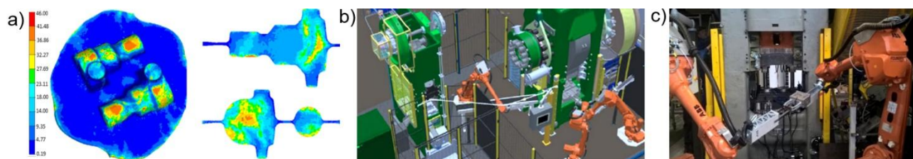
Figure 2 View: a) Final simulation results analysed forging process - distribution grains size, b) press forging line, c) photographs from the first industrial trials and system commissioning [2]
