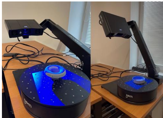
Figure 2 Scanning with GOM Scan 1 scanner setup with rotary table and ScanPort
