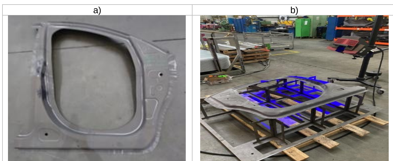
Figure 6 Photography of door ring sub-assembly after hot forming: a) drawpiece made on pilot line b) geometry inspection by using an optical scanner
