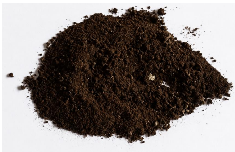
Figure 1. A sample of steelmaking dust prepared for hydrogen reduction
