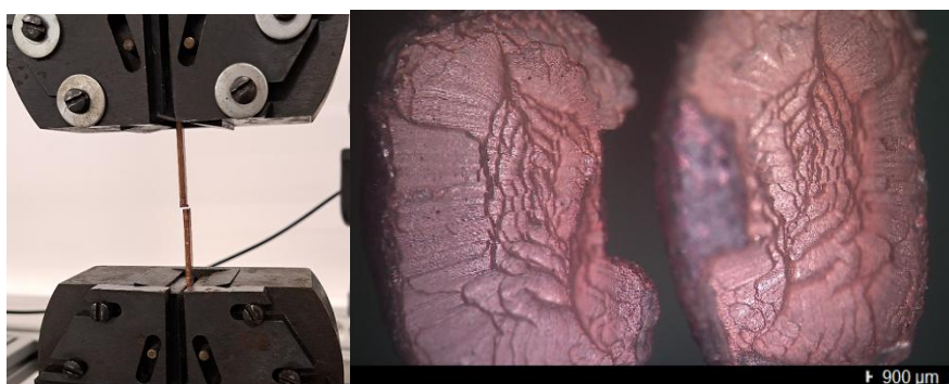
Figure 6 Fracture surface of the joint after tensile testing
