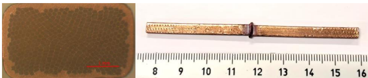
Figure 1 Structure of Cu-Nb 18% microcomposite conductor and welded joint
