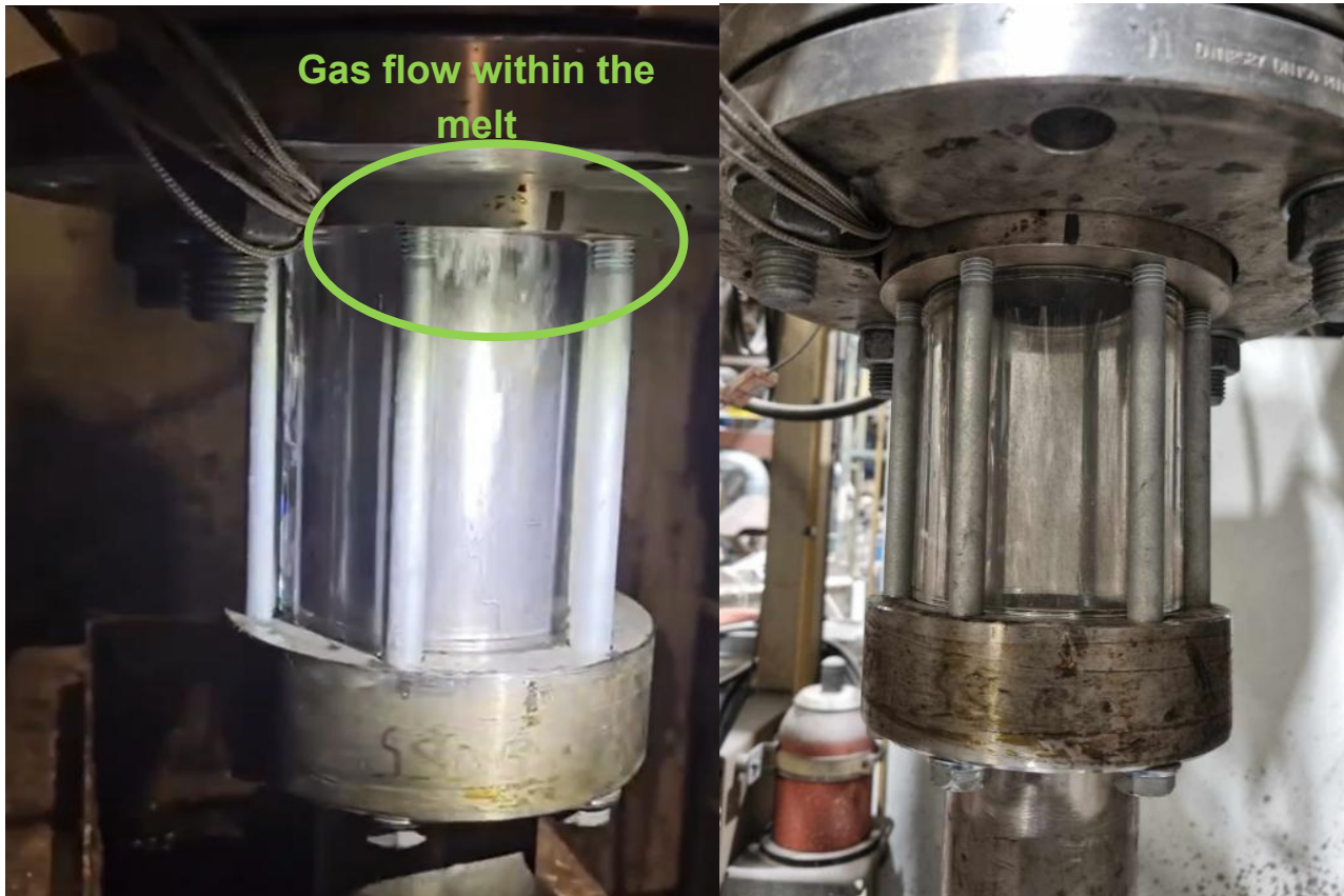
Figure 4 Glass window during (left) and after (right) the trials
