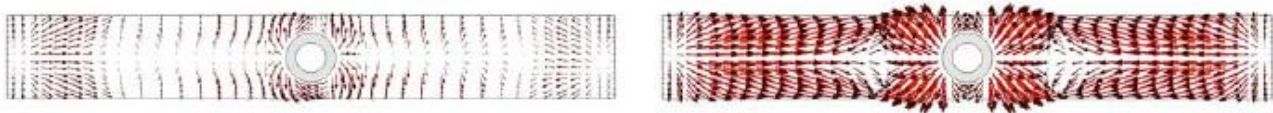
Figure 9 Meniscus metal flow velocities, no electromagnetic device ( left ), FC Mold accelerating the meniscus flow ( right ).
