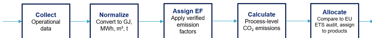
Figure 1 Methodology of modular CO 2 accounting for product-level Scope 1–2 emissions in BF–BOF steel production.
