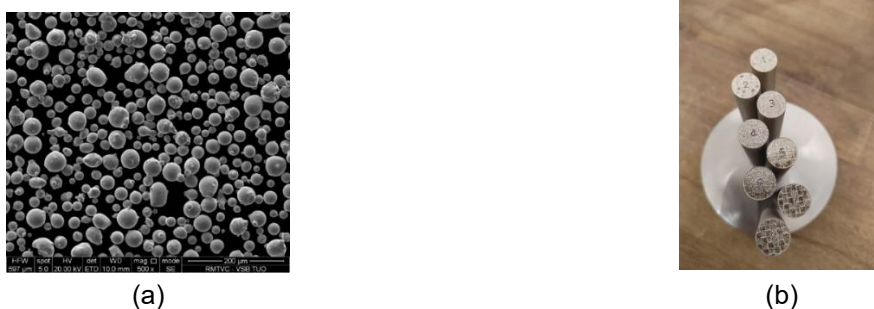
Figure 1 (a) SEM micrograph of input powder; (b) prepared rod samples in the building platform
