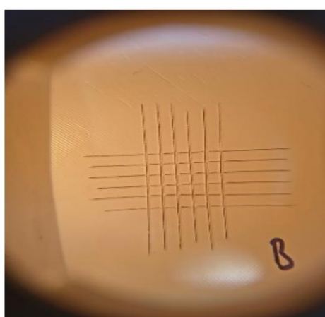
Figure 18 Cross-cut adhesion test for ASA sample: A top area classification 5, B bottom area classification 3
